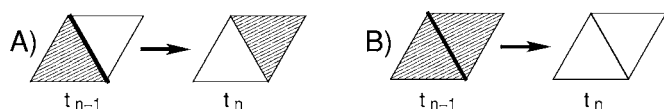
FIG. 1. Local dynamics of one update event. The imbalanced triads are represented as filled triangles, while the balanced ones as empty triangles. The shared link is represented as bold; this is the link involved in the update event. (a) When the update event flips the link shared by one imbalanced and one balanced triad we have diffusion. (b) When the update event flips the link shared by two imbalanced triads we have annihilation.
